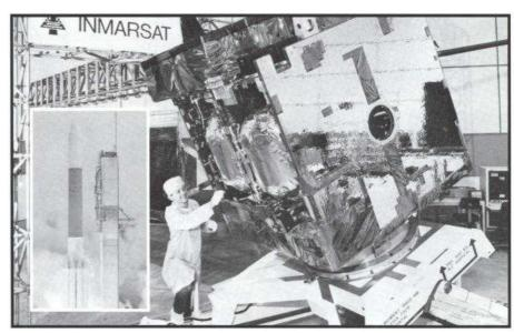
A British Aerospace engineer makes a routine check of the Inmarsat-2 satellite before its launch next month. The satellite will be carried aloft by a McDonnell Douglas Delta Rocket (at inset).
