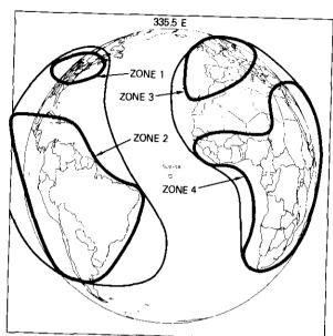
Figure 2. INTELSAT VI Hemi and Zone Antenna Coverage Contours for the AOR from Primary Satellite Location
