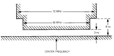
Figure 8b. INTELSAT TDMA RF Link Group Delay Response Limits
