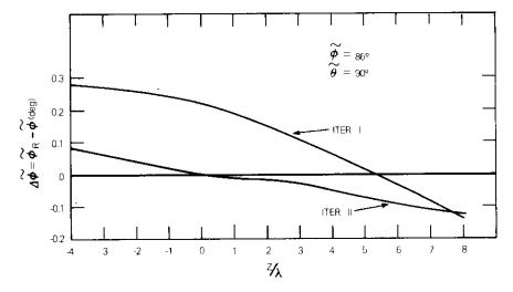
Figure 3. Beam Pointing Accuracy for the Feed on the CBDFL
