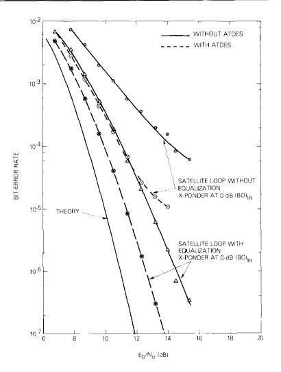
Figure 12. Satellite Loop Performance With and Without ATDES-BER vs  $E_b/N_o$
