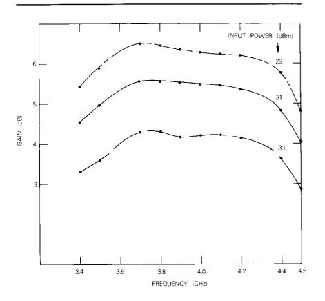
Figure 8. Measured Frequency Response of Balanced Amplifier
