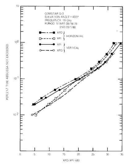
Figure 6. Cumulative Distributions of Measured XPD and XPI
