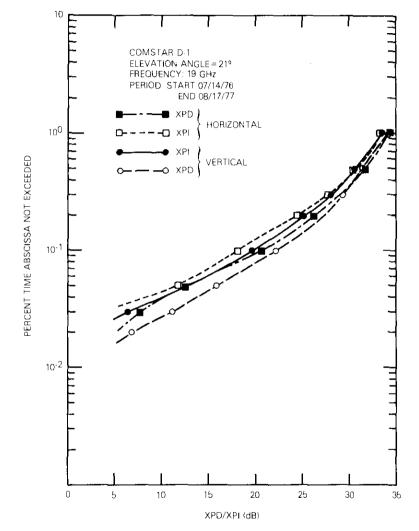
Figure 4. Cumulative Distributions of Measured XPD and XPI
