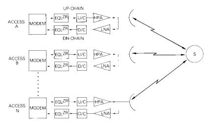
Figure 14. N-Access TDMA Configuration
