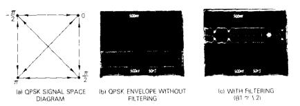
Figure 1. Effect of Band-Limiting PSK Signal
