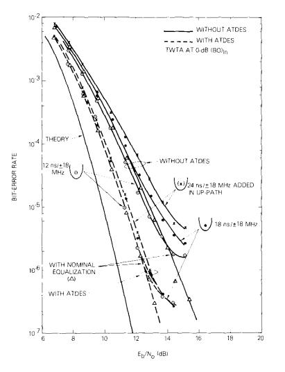
Figure 20. Channel Sensitivity Study With and Without ATDES— Parabolic Delay Distortion as Parameter
