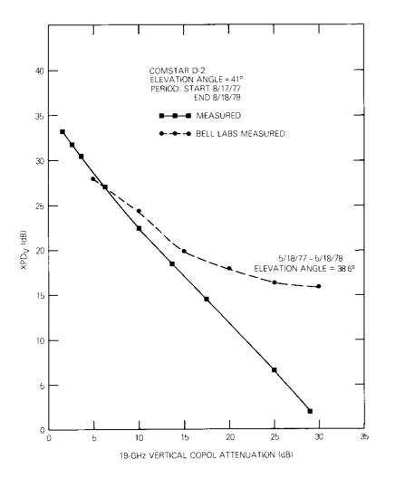
Figure 9. Comparison of Measured XPD with Bell Laboratories Data [3]
