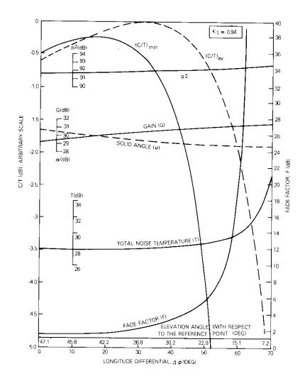
Figure 7. System Parameters vs Satellite Location for the Eastern United States
