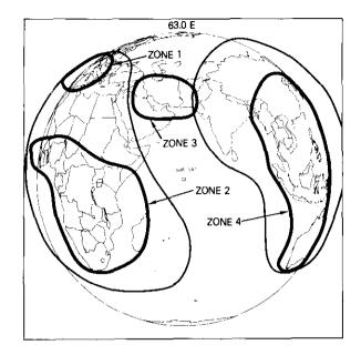
Figure 4. INTELSAT VI Hemi and Zone Antenna Coverage Contours for the IOR from Primary Satellite Location
