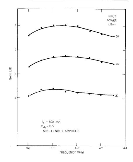
Figure 5. Measured Frequency Response of Single-Ended Amplifier
