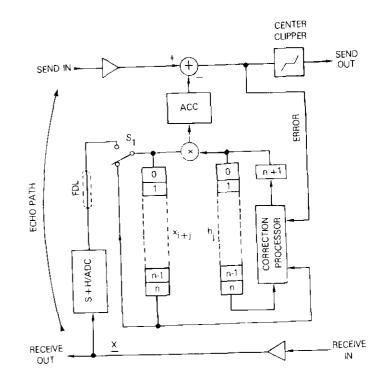
Figure 8. Digital Implementation of the Adaptive FIR Filter as Used in the Echo Canceller
