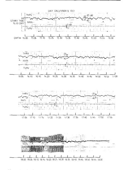
Figure 11. Ice Depolarization Event Recorded on December 9, 1977
