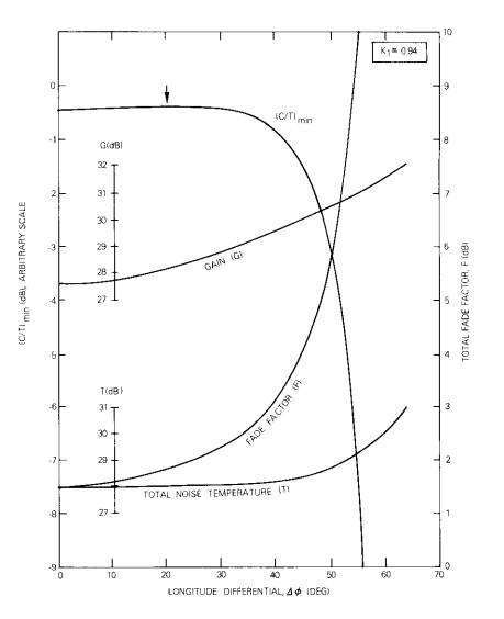
Figure 4. Minimum Performance for the Horizontal Elliptical Coverage Region
