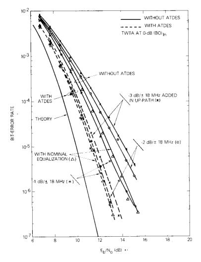
Figure 16. Channel Sensitivity Study With and Without ATDES— Amplitude Slope as Parameter
