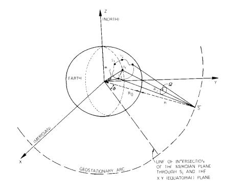
Figure 1. Geometry of Coverage by Satellite Antenna Beam
