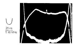
Figure 19. Link Equalization Perturbation Due to Parabolic Delay Distortion Added in Up-Path
