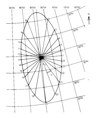
Figure 3b. Elliptical Coverage Region with Major Axis in the North-South Direction
