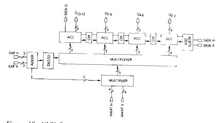
Figure 10. VLSI Convolution Processor (Floating-point multiplier and accumulator)
