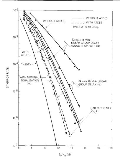
Figure 18. Channel Sensitivity Study With and Without ATDES— Linear Group Delay Distortion as Parameter
