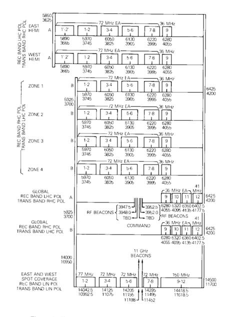
Figure 6. Transponder Center Frequencies, Bandwidths, and Polarization for INTELSAT VI
