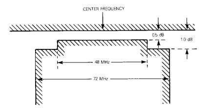
Figure 8a. INTELSAT TDMA RF Link Amplitude Response Limits
