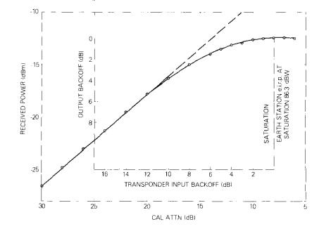
Figure 9. Satellite Transponder TWTA Power Transfer Curve
