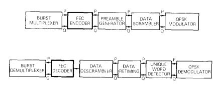
Figure 6. TDMA Terminal Interface for FEC Coding
