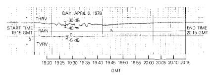
Figure 12. Ice Depolarization Event Recorded on April 6, 1978
