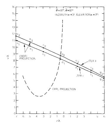
Figure 5. Projections on the yz-Plane of the CBDFL (solid lines) and of the Supplemental Line of Intersection of the OFPL and the Surface of Equation (22) (dotted line)
