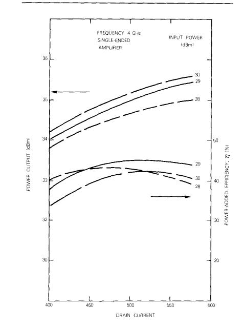
Figure 7. Output Power and Efficiency vs FET Drain Current of Single-Ended Amplifier at 4 GHz
