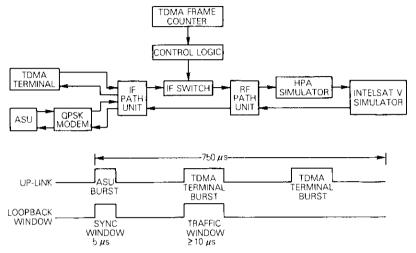
Figure 13. Simplified SS/TDMA Synchronization Test Configuration
