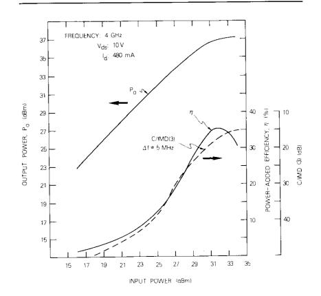
Figure 9. Output Power, Efficiency, and Intermodulation [C/IMD(3)] vs Input Power of Balanced Amplifier at 4 GHz
