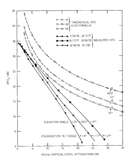
Figure 7. Comparisons of Measured XPD with CCIR-Predicted Result for Varying Elevation Angles
