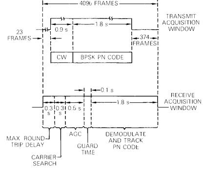
Figure 14. PN Acquisition Signal Format
