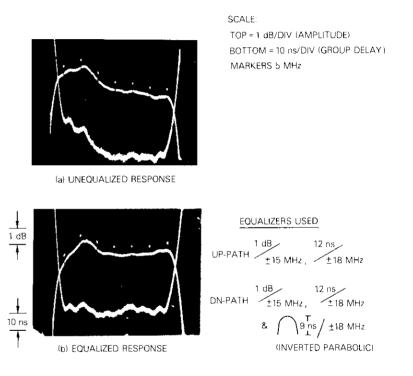
Figure 11. Satellite Loop Amplitude and Group Delay Response (6-dB TWTA Input Backoff)
