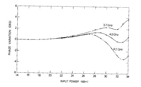
Figure 10. Phase Characteristics of Balanced Amplifier
