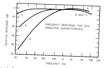
Figure 6. Frequency Response Characteristics for Sound Level Meters According to ANSI-S1.4-1971
