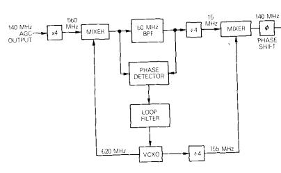
Figure 4. Carrier Recovery Circuit
