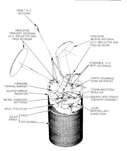
Figure 1. On-Orbit Configuration
