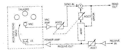
Figure 11. Echo Canceller with Automatic Gain Control Circuits
