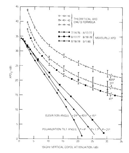
Figure 8. Comparisons of Measured XPD with Chu's Empirical Result [24] for Varying Elevation Angles
