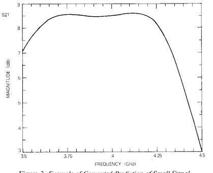
Figure 3. Example of Computed Prediction of Small Signal Gain-Frequency Response
