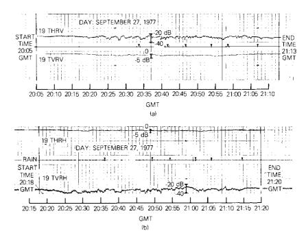
Figure 10. Ice Depolarization Event Recorded on September 27, 1977
