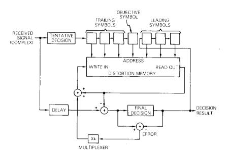
Figure 7. ATDES Processor Principle
