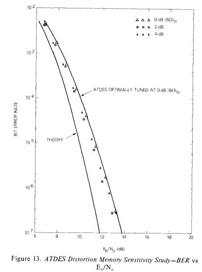
0-, 2-, and 4-dB input backoff operation as shown in Figure 13 indicates that the distortion memory is capable of improving the channel performance within the range of transponder operation expected in a 4/6-GHz band TDMA operating environment. In practice, the 2- and 4-dB performance curves (Figure 13) are somewhat better than the 0-dB curve. This improvement is attributed to the milder effect of the transponder nonlinearity at 2- and 4-dB input backoffs.
