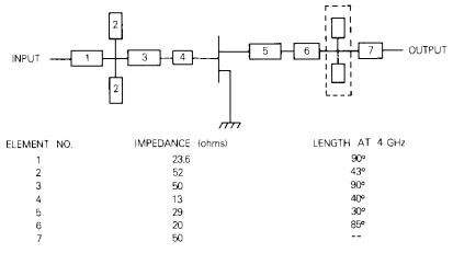
Figure 2. Schematic of the Input and Output Matching Networks
