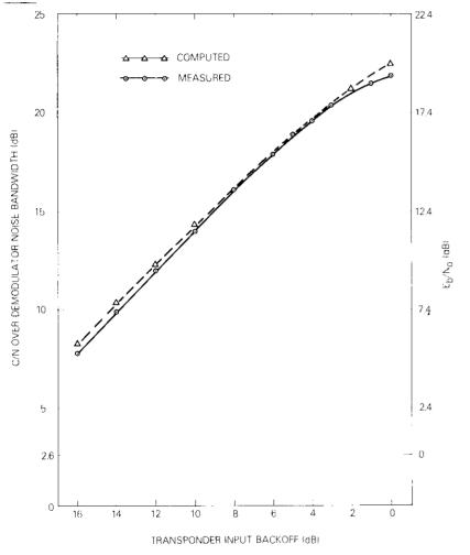
Figure 10. Link C/N and  $E_b/N_o$  vs Transponder Input Backoff
