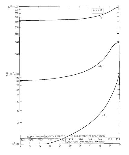
Figure 6. Noise Temperature vs Satellite Location for Eastern United States Coverage Region Figure 6 shows the dependence of the antenna and receiver noise temperature degradations  $\Delta T_1$  and  $\Delta T_2$  due to atmospheric absorption and rain fades, respectively (see Appendix A). The resultant total noise temperature,  $T_s$ , for the receive system is also shown. It is seen that, with
