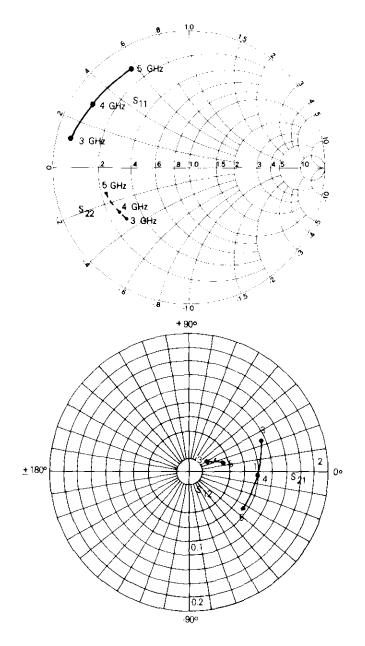
Figure 1. S-Parameters Used for Amplifier Design
