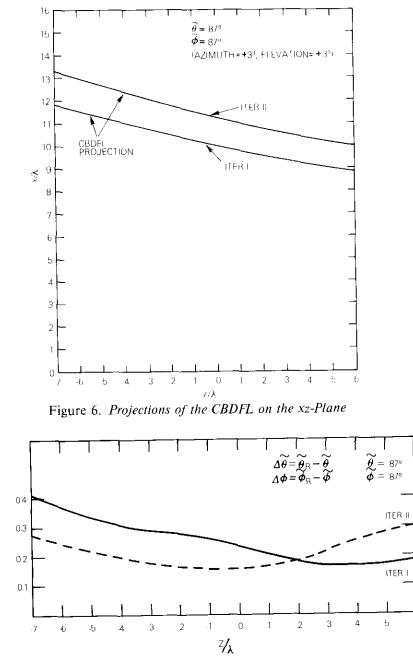
Figure 7. Beam Pointing Accuracy for the Feed on the CBDFL
