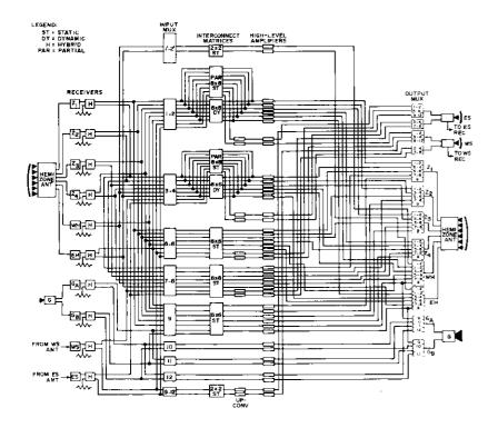
Figure 7. INTELSAT VI Simplified Signal Flow Diagram
